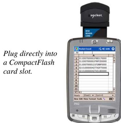
*Plug directly into a CompactFlash card slot.*
