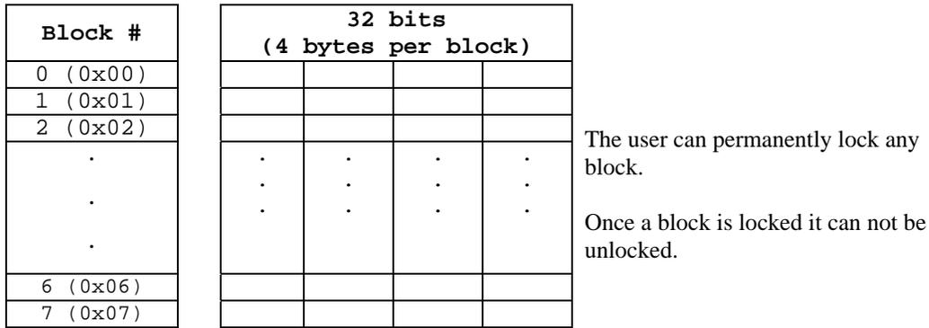
A 32-bit ID (factory programmed) uniquely identifies each Tag-it HF chip.
