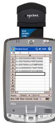
The CF RFID Reader Card is sleekly designed with no cables or batteries – it draws minimal power from the Pocket PC. The card is designed to withstand repeated three-foot drops to concrete – even when inserted in the Pocket PC.
