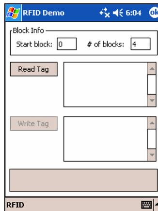
3. Hold the Pocket PC in the correct position to read RFID tags — parallel to the tag and directly above it, at most 2.0 inches above. Tap Read Tag.
